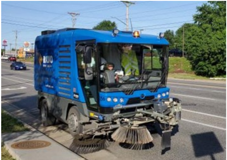
Street sweeping is part of the City’s ongoing pollution reduction practices. This practice helps reduce sediment and debris from entering the MS4 and the City’s streams.
